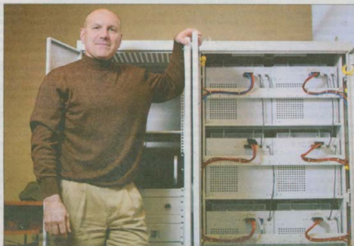
Sam Reiney/DJC Michael Morse, vice president of operations for Powin Energy, stands in front of a single-phase Powin Energy product able to store 16 kilowatt-hours of electrical energy.
